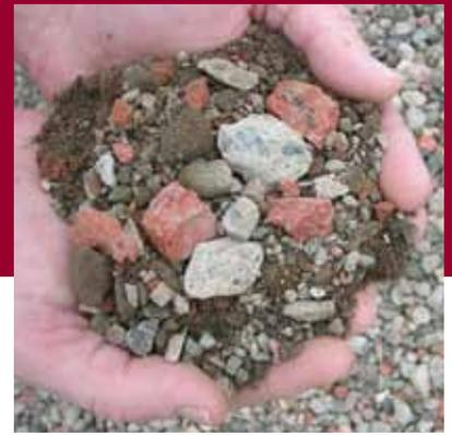
Alex Fraser's 20mm Class 4 Crushed Concrete is a popular recycled product that is easy to compact and trim. There are sound reasons for using Alex Fraser's 20mm Class 4 Crushed Concrete on your next project.
